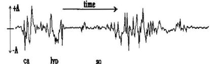
The horizontal axis ("time") represents the passage of time, and the vertical axis ("A" to "+A") represents the strength of the sound's signal at that specific instant in time. When you digitize a waveform, you measure the vertical deflection of the wave at very short intervals of time, creating a discrete table of values representing the approximate (within the limits of error allowed by the sampling intervals) shape of the wave.
